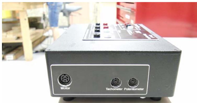
Figure 2: Servo Motor Interface
