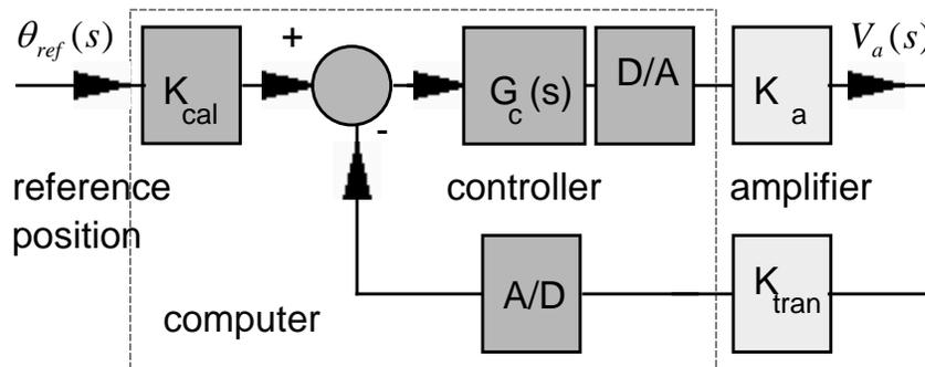
Figure 5: Block Diagram of the Servomotor and Computer
