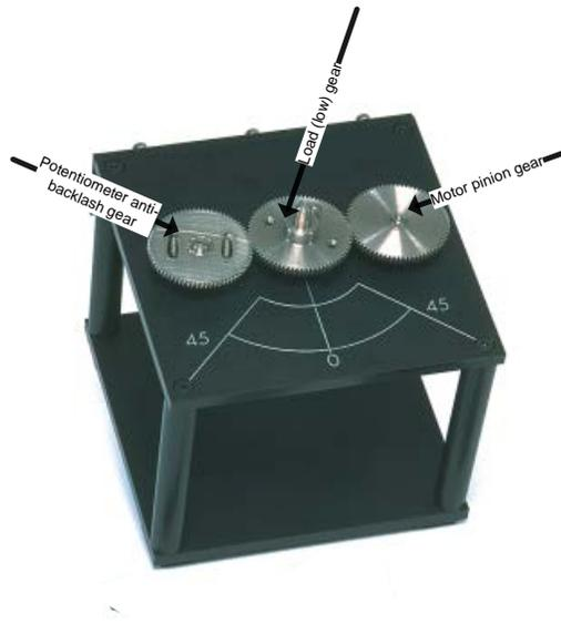
Figure 1: Servo Motor Components
