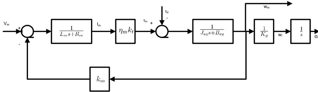
Figure 4: Block Diagram of the DC Motor
