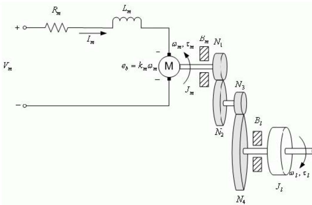
Figure 3: Schematic Diagram of the Armature Controlled DC Motor
