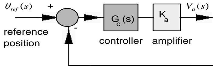
Figure 6: Equivalent Unity Feedback Block Diagram of the Servomotor System
