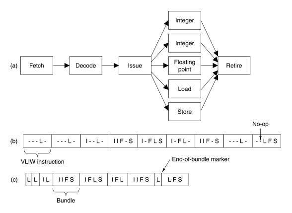
**Figure 8-2.** (a) A CPU pipeline. (b) A sequence of VLIW instructions. (c) An instruction stream with bundles marked.
