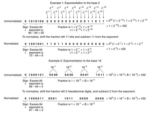
**Figure B-3.** Examples of normalized floating-point numbers.
