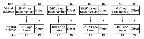
Figure 6-17. Virtual to physical mappings on the UltraSPARC.
