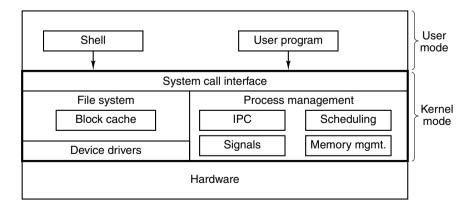
Figure 6-30. The structure of a typical UNIX system.
