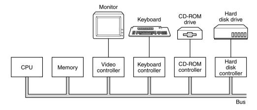
Figure 2-29. Logical structure of a simple personal computer.
