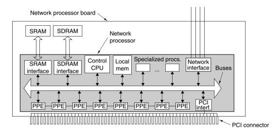
Figure 8-15. A typical network processor board and chip.
