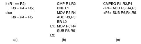
Figure 5-53. (a) An if statement. (b) Generic assembly code for (a). (c) Predicated execution.
