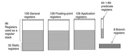
Figure 5-49. The Itanium 2's registers.
