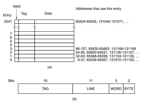
Figure 4-38. (a) A direct-mapped cache. (b) A 32-bit virtual address.
