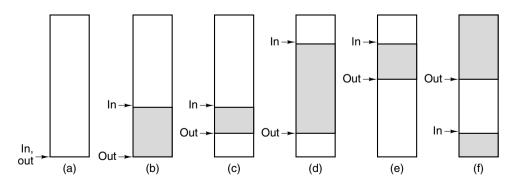
Figure 6-24. Use of a circular buffer.
