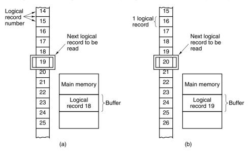
**Figure 6-19.** Reading a file consisting of logical records. (a) Before reading record 19. (b) After reading record 19.
