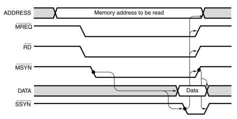
Figure 3-39. Operation of an asynchronous bus.
