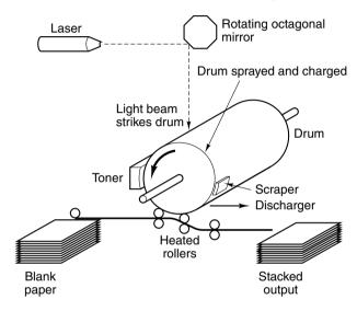
Figure 2-35. Operation of a laser printer.
