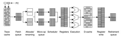
**Figure 8-9.** Resource sharing between threads in the Pentium 4 NetBurst microarchitecture.
