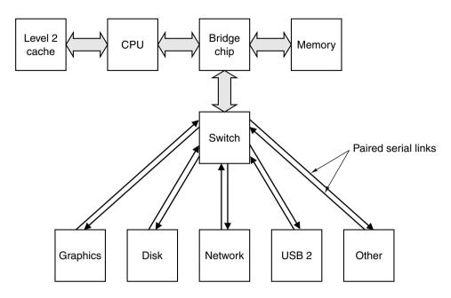
Figure 3-57. A typical PCI Express system.
