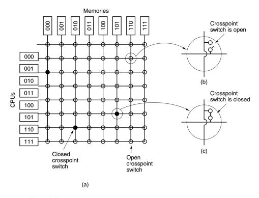
**Figure 8-27.** (a) An  $8 \times 8$  crossbar switch. (b) An open crosspoint. (c) A closed crosspoint.
