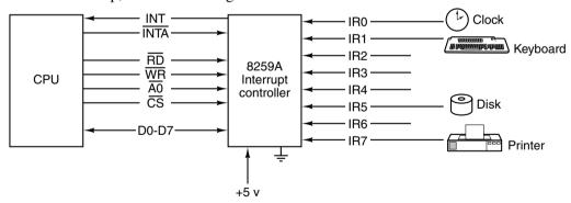
Figure 3-43. Use of the 8259A interrupt controller.
