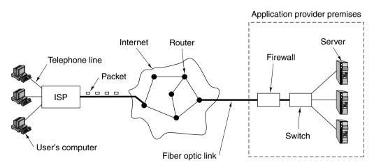
**Figure 8-13.** How users are connected to servers on the Internet.
