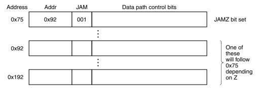
**Figure 4-7.** A microinstruction with JAMZ set to 1 has two potential successors.
