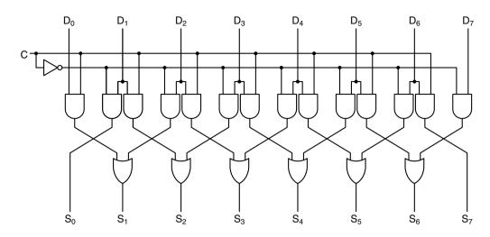
Figure 3-16. A 1-bit left/right shifter.
