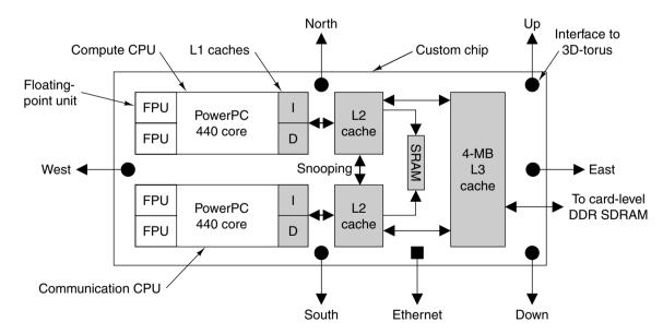
Figure 8-36. The BlueGene/L custom processor chip.
