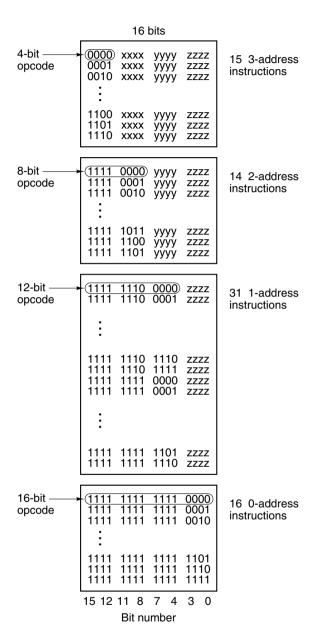
**Figure 5-13.** An expanding opcode allowing 15 three-address instructions, 14 two-address instructions, 31 one-address instructions, and 16 zero-address instructions. The fields marked *xxxx*, *yyyy*, and *zzzz* are 4-bit address fields.
