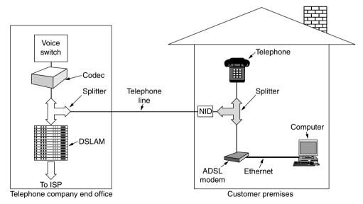
Figure 2-39. A typical ADSL equipment configuration.
