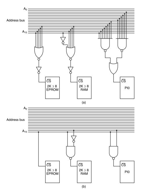
Figure 3-62. (a) Full address decoding. (b) Partial address decoding.
