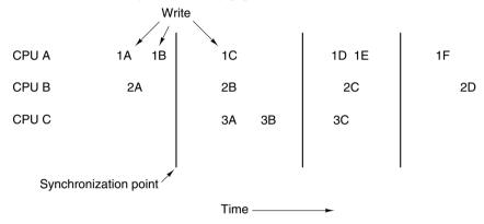
**Figure 8-23.** Weakly consistent memory uses synchronization operations to divide time into sequential epochs.
