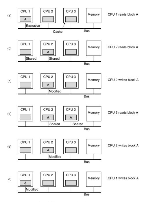
Figure 8-26. The MESI cache coherence protocol.
