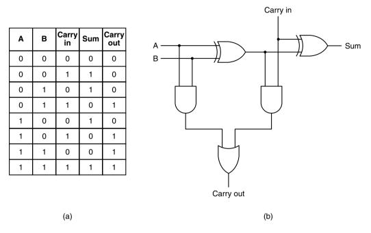
Figure 3-18. (a) Truth table for full adder. (b) Circuit for a full adder.
