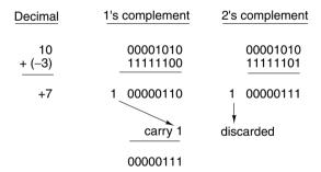
Figure A-9. Addition in one's complement and two's complement.
