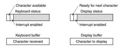
Figure 5-31. Device registers for a simple terminal.
