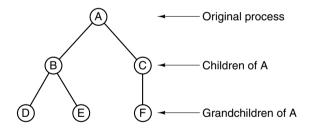
Figure 6-42. A process tree in UNIX.
