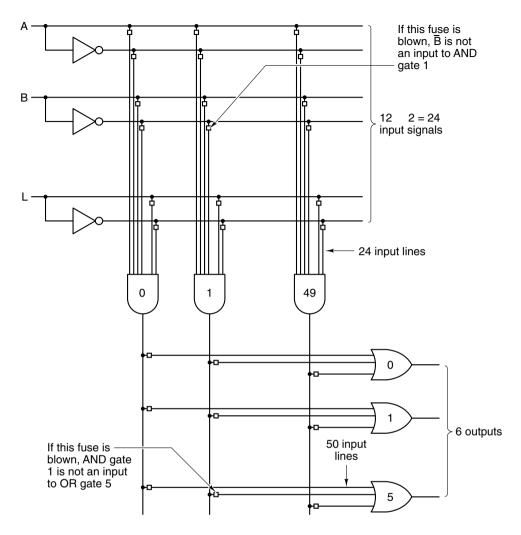
**Figure 3-15.** A 12-input, 6-output programmable logic array. The little squares represent fuses that can be burned out to determine the function to be computed. The fuses are arranged in two matrices: the upper one for the AND gates and the lower one for the OR gates.
