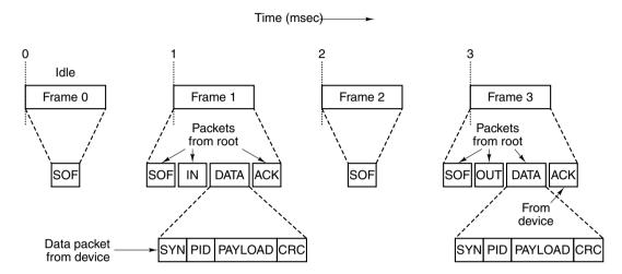
Figure 3-59. The USB root hub sends out frames every 1.00 msec.
