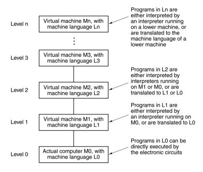
Figure 1-1. A multilevel machine.
