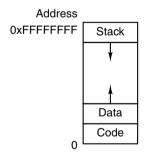
**Figure 6-32.** The address space of a single UNIX process.
