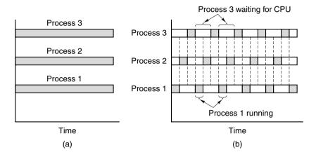
**Figure 6-23.** (a) True parallel processing with multiple CPUs. (b) Parallel processing simulated by switching one CPU among three processes.
