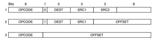
Figure 5-25. A simple design for the instruction formats of a three-address machine.
