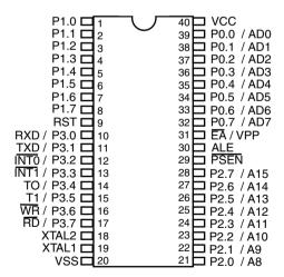
**Figure 3-49.** Physical pinout of the 8051.
