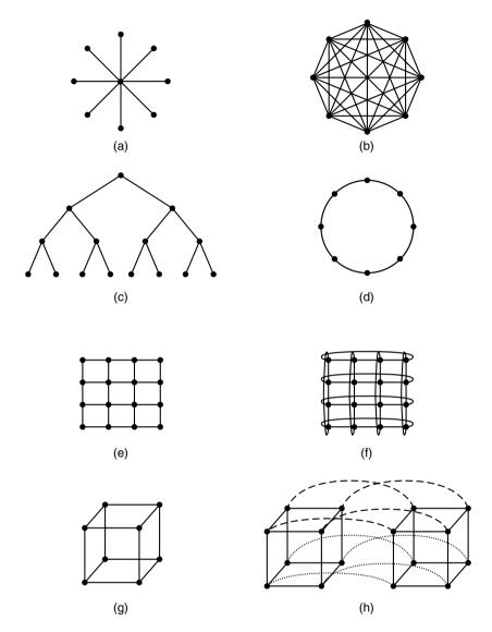
**Figure 8-35.** Various topologies. The heavy dots represent switches. The CPUs and memories are not shown. (a) A star. (b) A complete interconnect. (c) A tree. (d) A ring. (e) A grid. (f) A double torus. (g) A cube. (h) A 4D hypercube.
