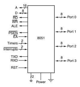
**Figure 3-50.** Logical pinout of the 8051.
