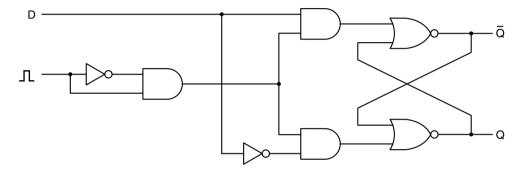
Figure 3-26. A D flip-flop.
