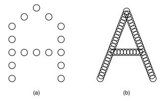
**Figure 2-34.** (a) The letter "A" on a  $5 \times 7$  matrix. (b) The letter "A" printed with 24 overlapping needles.
