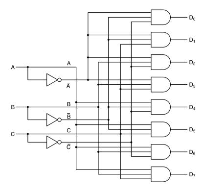
Figure 3-13. A 3-to-8 decoder circuit.
