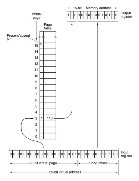
Figure 6-4. Formation of a main memory address from a virtual address.
