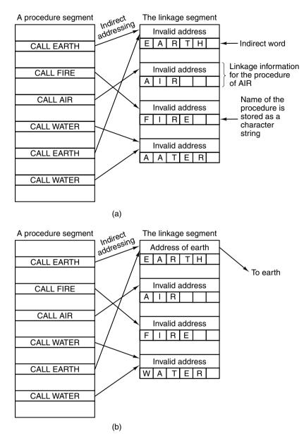
**Figure 7-18.** Dynamic linking. (a) Before *EARTH* is called. (b) After *EARTH* has been called and linked.
