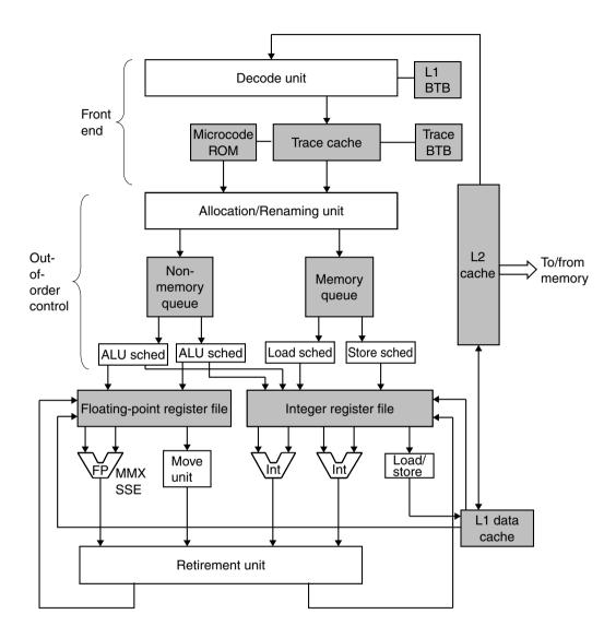
Figure 4-47. A simplified view of the Pentium 4 data path.
