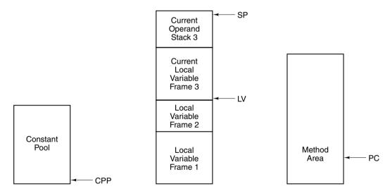
Figure 4-10. The various parts of the IJVM memory.
