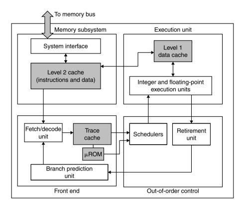
**Figure 4-46.** The block diagram of the Pentium 4.
