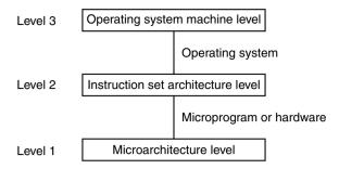
**Figure 6-1.** Positioning of the operating system machine level.
