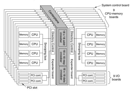
Figure 8-32. The Sun Microsystems E25K multiprocessor.
