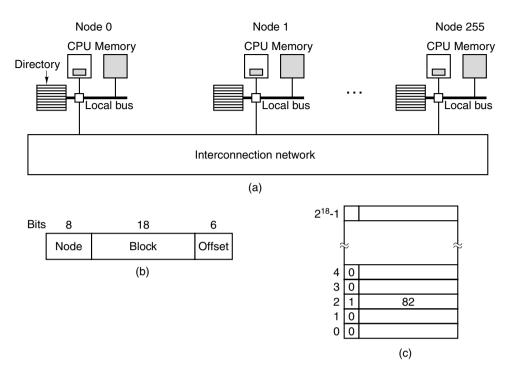
**Figure 8-31.** (a) A 256-node directory-based multiprocessor. (b) Division of a 32-bit memory address into fields. (c) The directory at node 36.
