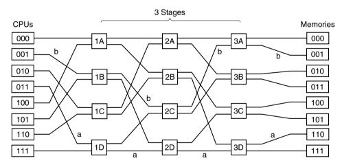
Figure 8-29. An omega switching network.
