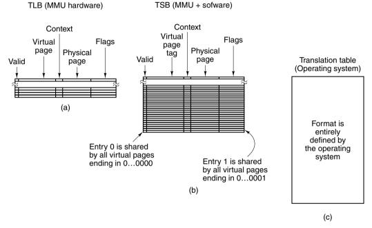
**Figure 6-18.** Data structures used in translating virtual addresses on the UltraSPARC. (a) TLB. (b) TSB. (c) Translation table.
