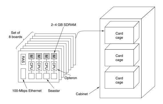
Figure 8-38. Packaging of the Red Storm components.
