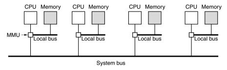
**Figure 8-30.** A NUMA machine based on two levels of buses. The Cm\* was the first multiprocessor to use this design.
