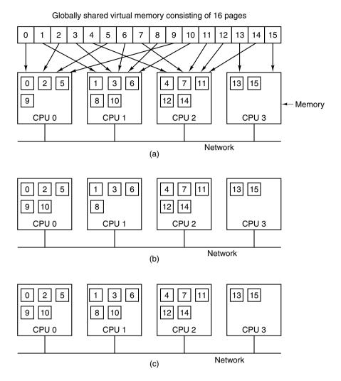
**Figure 8-44.** A virtual address space consisting of 16 pages spread over four nodes of a multicomputer. (a) The initial situation. (b) After CPU 0 references page 10. (c) After CPU 1 references page 10, here assumed to be a read-only page.
