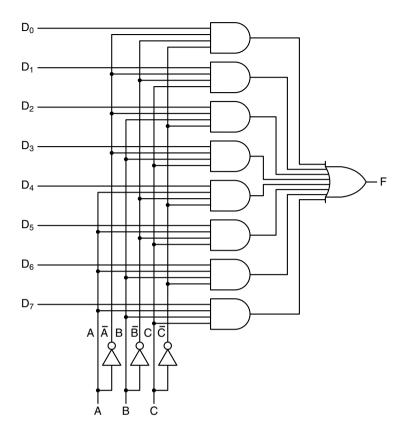
Figure 3-11. An eight-input multiplexer circuit.
