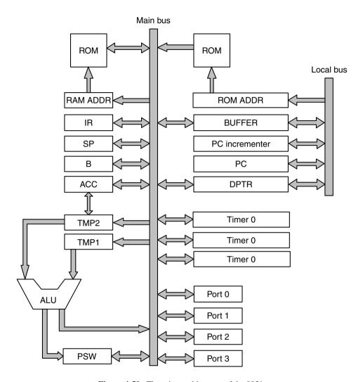
Figure 4-50. The microarchitecture of the 8051.
