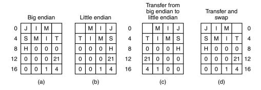
**Figure 2-12.** (a) A personnel record for a big endian machine. (b) The same record for a little endian machine. (c) The result of transferring the record from a big endian to a little endian. (d) The result of byte-swapping (c).
