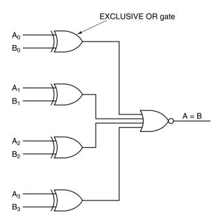
Figure 3-14. A simple 4-bit comparator.
