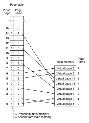
**Figure 6-5.** A possible mapping of the first 16 virtual pages onto a main memory with eight page frames.
