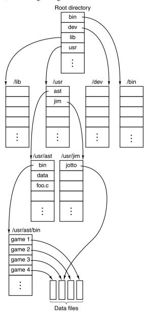
Figure 6-36. Part of a typical UNIX directory system.
