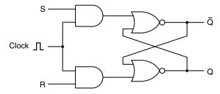
Figure 3-23. A clocked SR latch.
