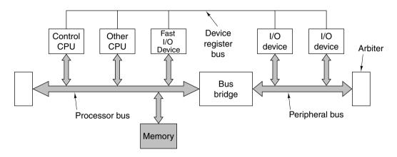
Figure 8-12. An example of the IBM CoreConnect architecture.
