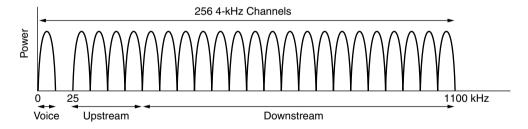
Figure 2-38. Operation of ADSL.
