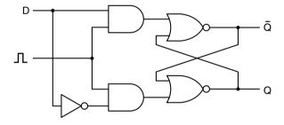
Figure 3-24. A clocked D latch.
