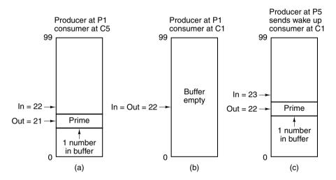
Figure 6-26. Failure of the producer-consumer communication mechanism.
