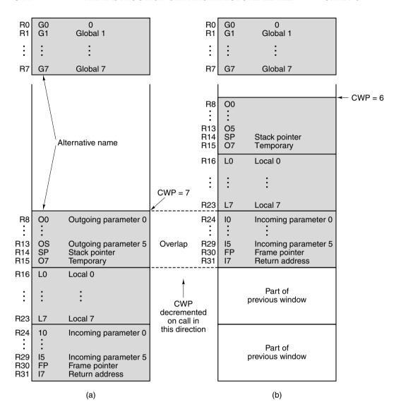
Figure 5-5. Operation of the UltraSPARC III register windows.
