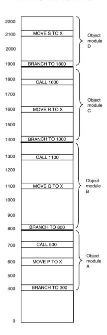
**Figure 7-17.** The relocated binary program of Fig. 7-15(b) moved up 300 addresses. Many instructions now refer to an incorrect memory address.
