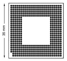
Figure 3-44. The Pentium 4 physical pinout.
