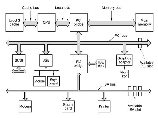
**Figure 3-52.** Architecture of an early Pentium system. The thicker buses have more bandwidth than the thinner ones but the figure is not to scale.
