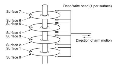
Figure 2-20. A disk with four platters.
