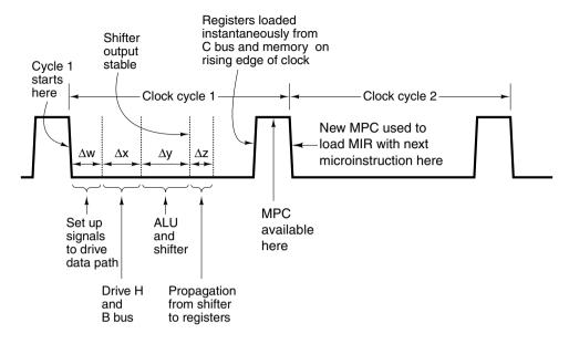
Figure 4-3. Timing diagram of one data path cycle.
