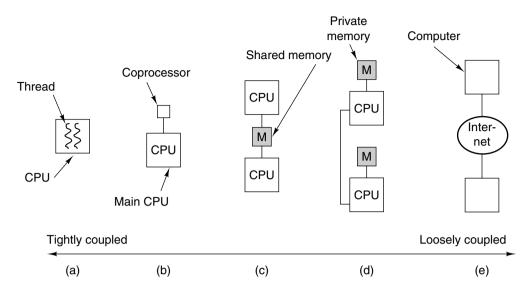
**Figure 8-1.** (a) On-chip parallelism. (b) A coprocessor. (c) A multiprocessor. (d) A multicomputer. (e) A grid.
