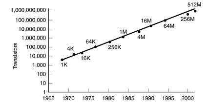
**Figure 1-8.** Moore's law predicts a 60-percent annual increase in the number of transistors that can be put on a chip. The data points given in this figure are memory sizes, in bits.
