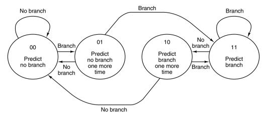
Figure 4-42. A 2-bit finite-state machine for branch prediction.
