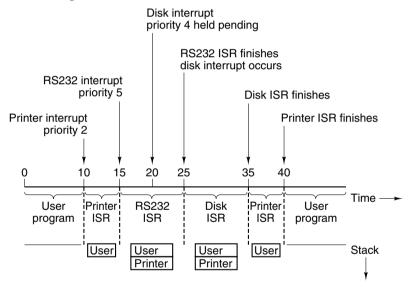
Figure 5-46. Time sequence of multiple interrupt example.
