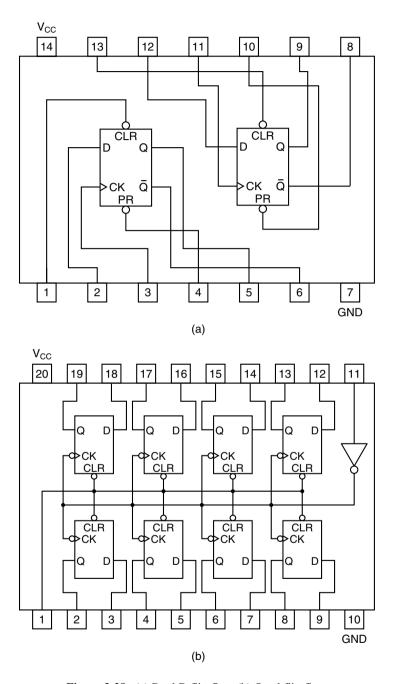
Figure 3-28. (a) Dual D flip-flop. (b) Octal flip-flop.
