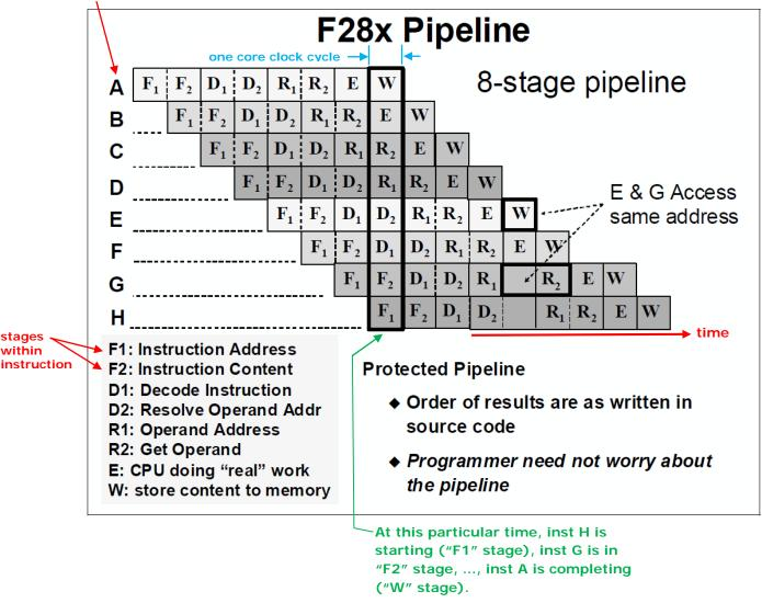
Note that the Harvard architecture allows instructions to be fetched at the same time operations are performed on the data.
