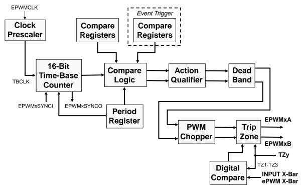
Figure 1. Enhanced Pulse Width Modulator (ePWM) Module Block Diagram
